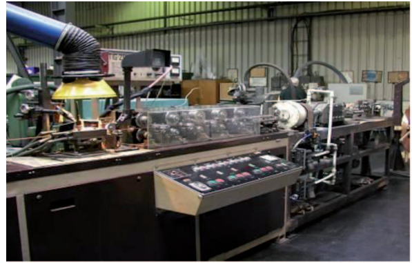
Fig. 3. Technological line for fabrication of composites (semi-products) used for the production of bimetallic wires
