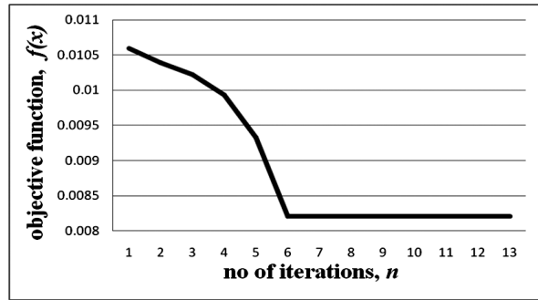
Figure 4. The objective function, f(x) with respect to the number of iterations, n for the SPSO algorithm for P2.
