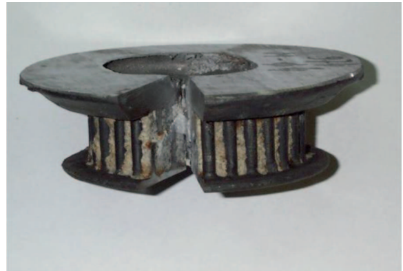
Fig. 2. The point of sample cutting from ingot top – filter poured with steel, for metallographic tests
