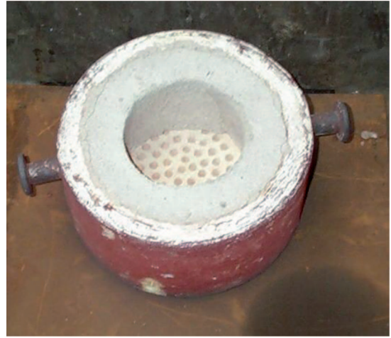
Fig. 1. Hot top with installed filter. Channel diam. 4 mm
