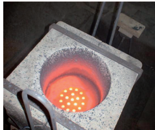
Fig. 7. Hot top with filter following completed casting process
