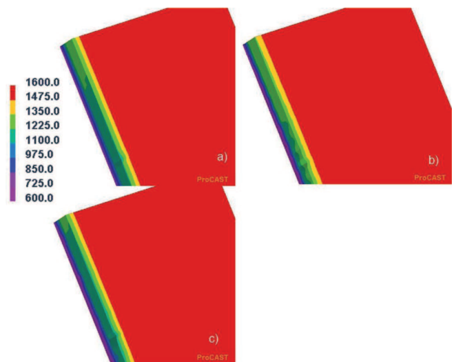
Fig. 5. The temperature distribution (°C) for: a) the reference parameters, b) increased casting speed, c) increased the intensity of cooling
