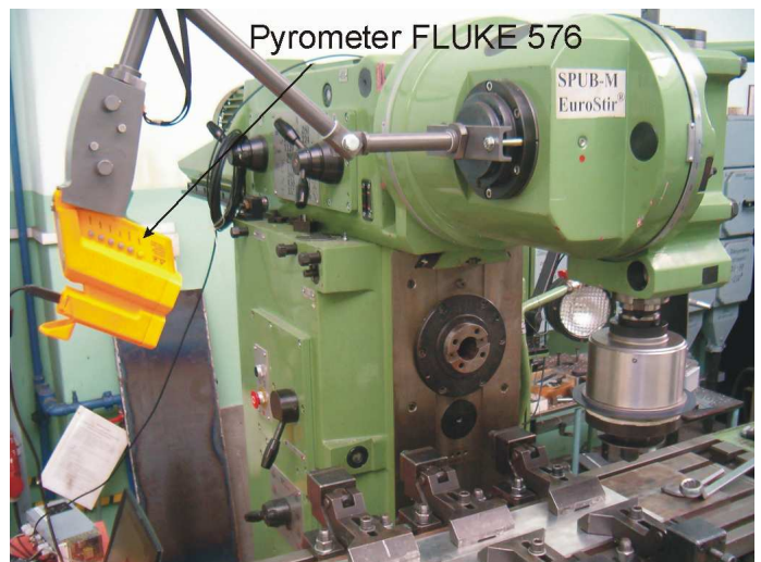
Fig. 3. Station for the temperature measurements of welding region: FLUKE 576 pyrometer used for measuring of temperature of weld face surface
