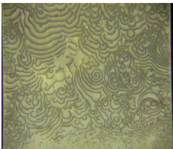
Fig. 5. Optical image of a Ag-In coating; 0.4 \text{ A dm}^{-2} , 35 min, electrolyte composition: 0.15 M In, 0.06 M Ag, 0.5 M KCN and 0.1 M D(+)-Glucose. Width of the sample – 1 cm
