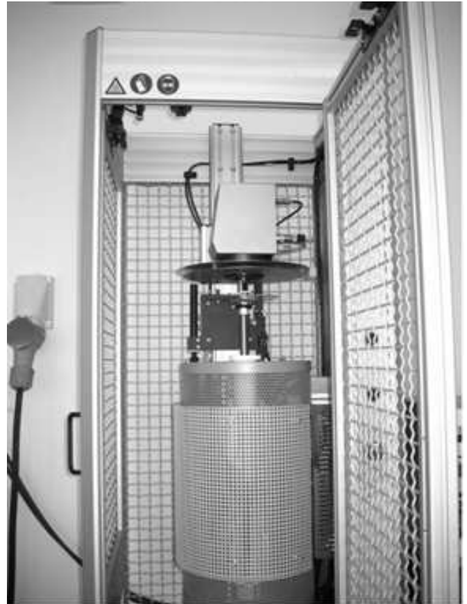
Fig. 3. The high-temperature rheometer FRS1600 used in this research
