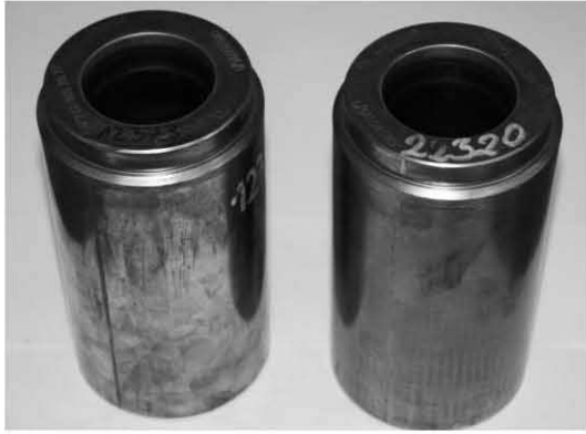
Fig. 10. Optimized tools for forging CVJ casing
