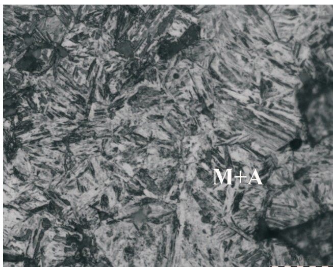
Fig. 3. Micrograph of Astaloy CrM-based PM steel sintered at 1120°C in H 2 ; martensite (M) in austenite (A) matrix; mag. 500x
