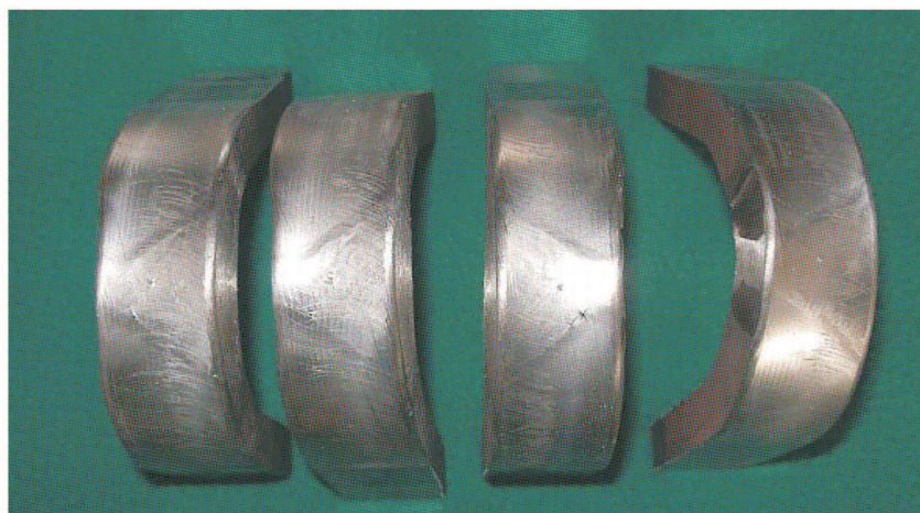
Fig. 5. Samples after side bend test of butt joint of pipes made of PB2 steel
