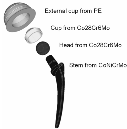
Fig. 7. Modeled exemplary constructional solution of cemented endoprostheses: stem from CoNiCrMo, head from Co28Cr6Mo Ø28 mm, two-layered cup Co28Cr6Mo-PE.
