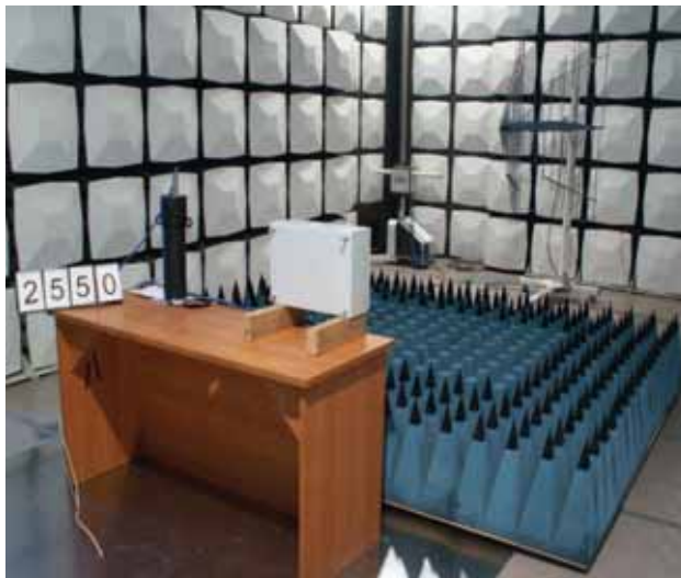
Fig. 2. Device prepared for radiated radio-frequency electromagnetic field immunity test
