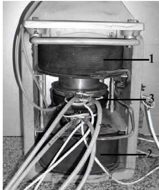
Fig. 1. Device for thermal annealing of ring-shaped cores in transversal magnetic field: 1, 2 – magnet polepieces, 3 – furnace with ring-shaped core
