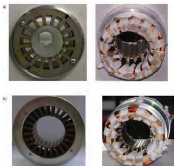
Fig. 1. The view of bearingless motor stators: a) 2-phase; b) 3-phase
