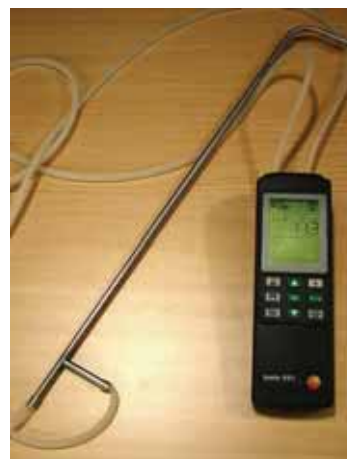
Fig. 4. Digital micro manometer TESTO 521 cooperating with Prandtl tube
