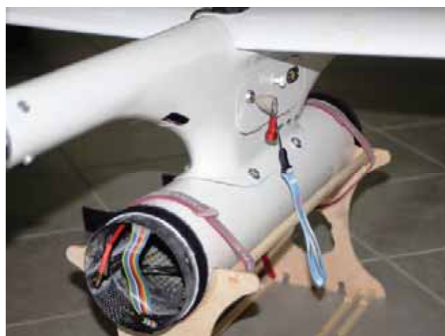
Fig. 11. Under-fuselage storage for avionics equipment
