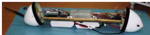
Fig. 10. Storage tray with mounted on-board devices
