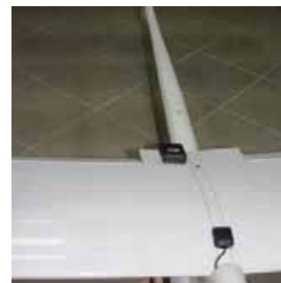
Fig. 12. GPS antenna and GPS tracker mounted on upper skin of center-wing
