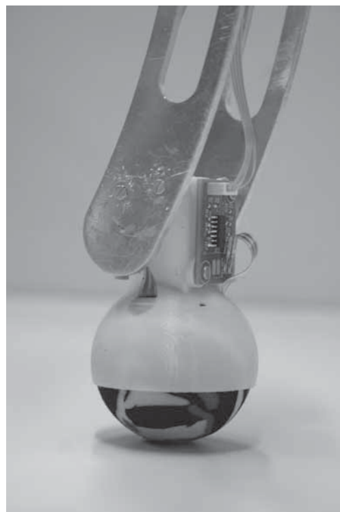
Fig. 1. A new design of the Messor robot foot equipped with the force measurement sensors
