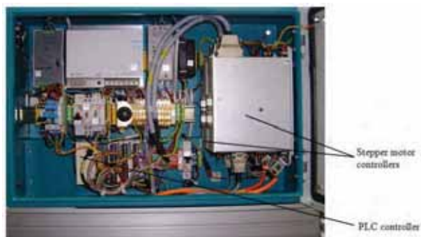
Fig. 2. View on the arrangement of elements of the control system in the control panel of the multifunctional tester for electronically protected documents
