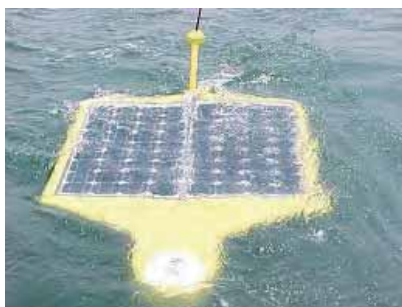
Rys. 20. Robot Solar AUV (Autonomous Undersea Systems Institute) Fig. 20. Solar AUV robot (Autonomous Undersea Systems Institute)
