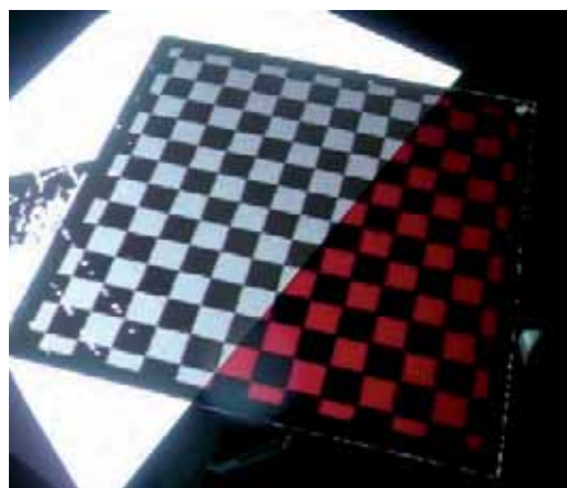
Fig. 1. A black and white pattern projected by the calibrated projector onto the physical chessboard partially covered by a sheet of paper
