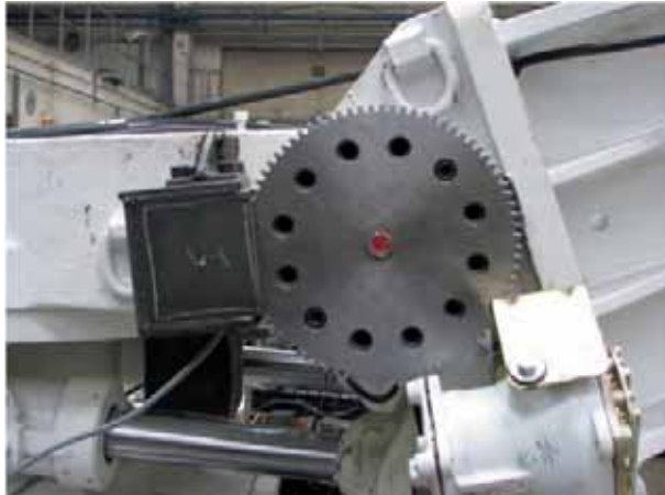
Fig. 9. Installation of jib position sensor [4]
