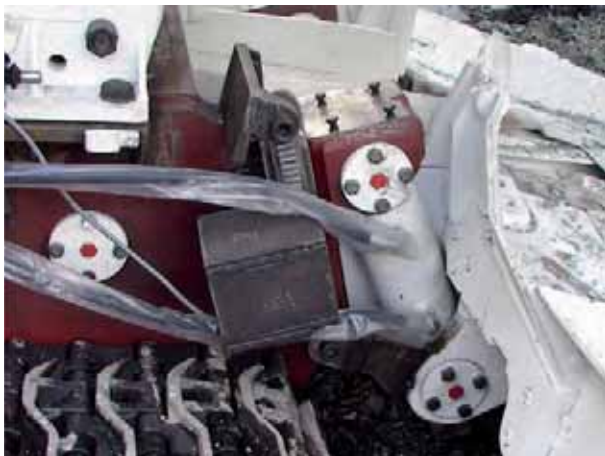
Fig. 10. Installation of loading table position sensor [4]
