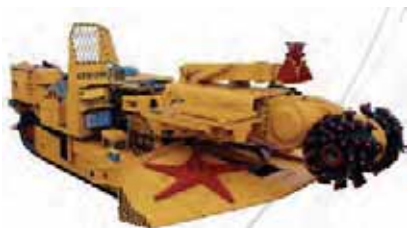
Fig. 3. KTW-200 roadheader manufactured by WAMAG [12]
