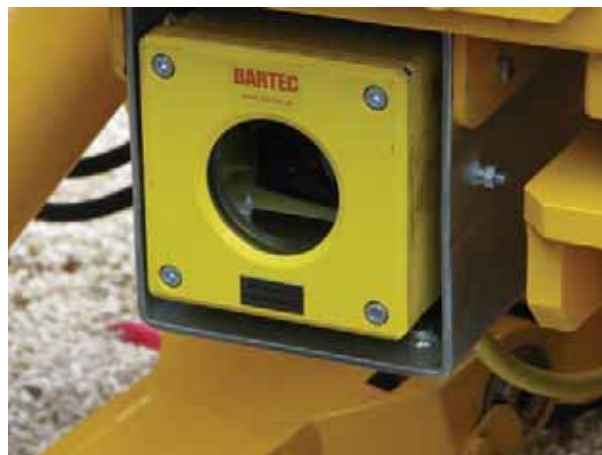
Fig. 5. Laser system for positioning of KTW 150 roadheader [own source – Mining Fair 2011]
