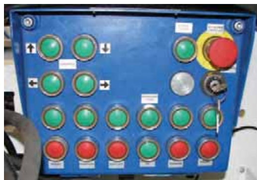
Fig. 1. Desk of operator of R-130 roadheader [own source – Mining Expo 2008]
