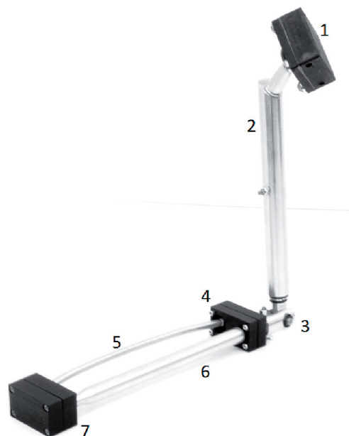
Fig. 1. Photography of prototype bone system: 1 – articulatio humeri, 2 – humerus, 3 – hinge elbow joint (humeroulnar and humeroradial), 4 – proximal radioulnar joint, 5 – radius, 6 – ulna, 7 – distal radioulnar joint
