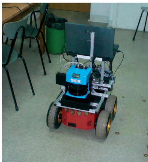
Fig. 1. Robot PIONEER 3AT equipped with 3D laser measurement system
