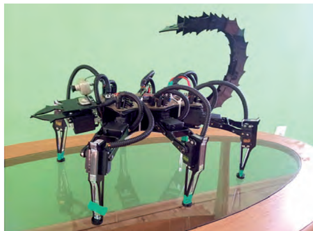
Fig. 1. View of the built walking six-feet mobile robot (hexapod)
