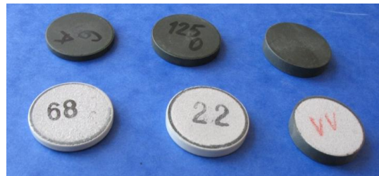
Fig. 1. Varistor samples: ZnO structures after being fired (top row) and with metalized contacts (bottom row); the thickness of the varistor structure determines the voltage value when the varistor begins to conduct current: left – 280 V, middle – 440 V, right – 660 V.
