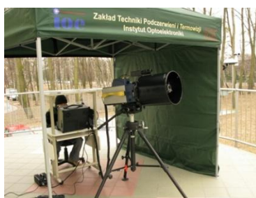
Fig. 1. HyperCam sensor during the measurement.
