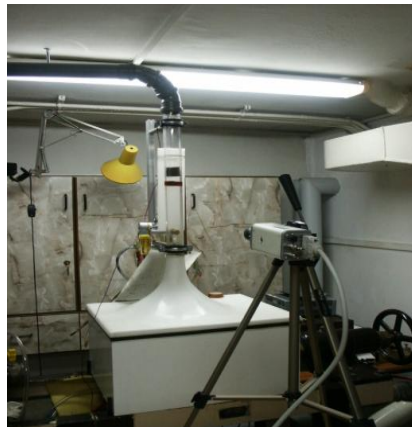
Fig. 6. Flow visualization measuring stand.
