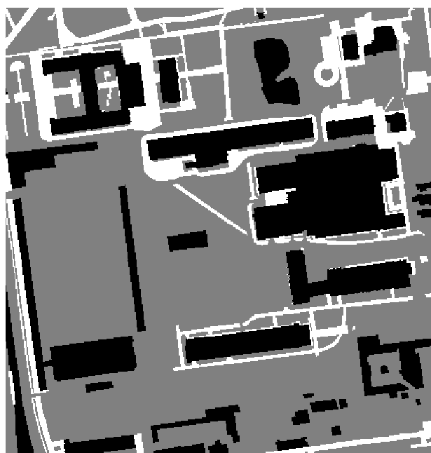
Fig. 6. A raster map of the University campus. White, grey, black correspond to preferred, probable and forbidden regions respectively.
