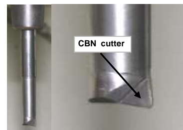
Fig. 2. CBN end mill applied in the research
