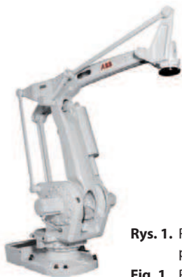
Fig. 1. Robot ABB IRB 660 dedicated to palletizing
