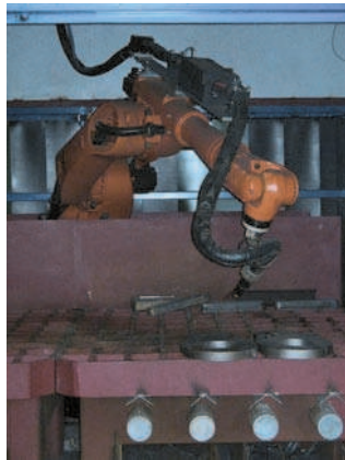
Fig. 3. Robotized cell for beveling with plasma cutting technology and use of KR 60 KUKA robot
