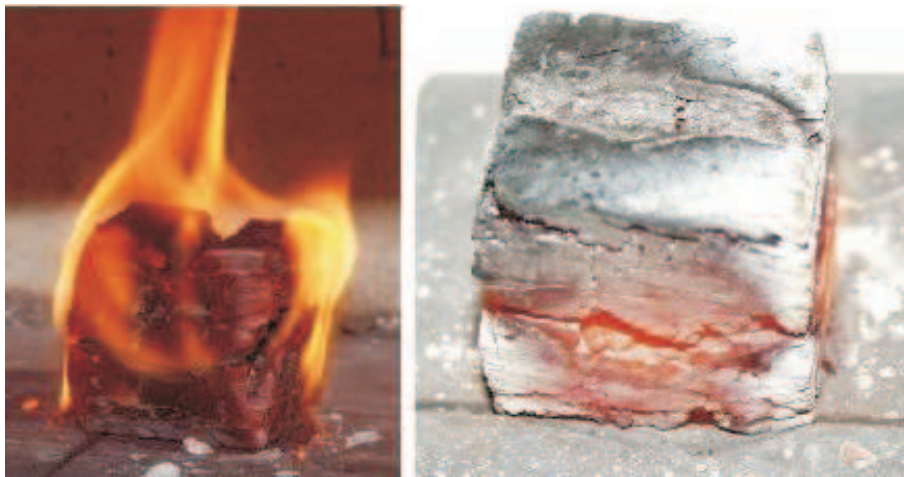
Figure 6. Combustion of volatile matter and char particles during tests on the fracture toughness rate.
