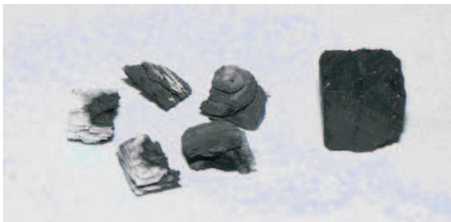
Figure 3. Delamination of coal particles after 60 s of combustion process.
