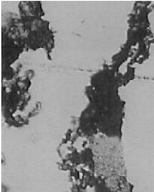
Fig. 7. Particles of ultimate wear, they have pitting on the surface caused by repeated passage of zone of rolling contact, and they are produced at the end of fatigue wear. Magnification 500x
