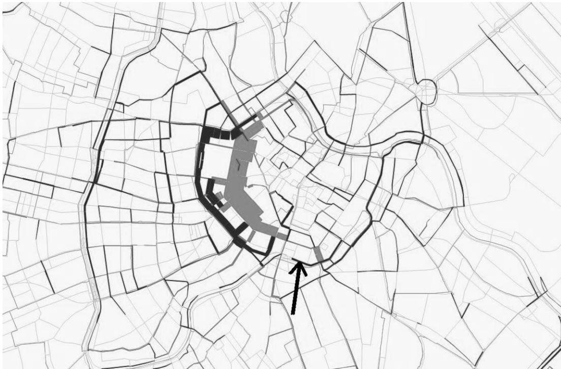
Fig. 8. Differential net of pre- and during-EURO 2008 traffic; light grey = decrease, dark grey = increase, black arrow = log point
