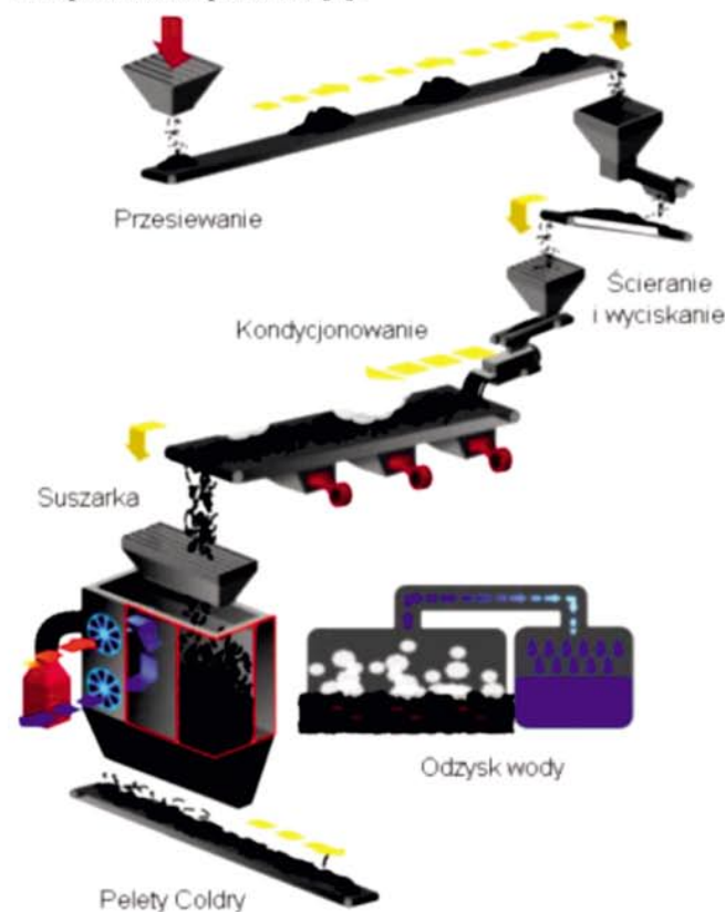
Rys. 11. Schemat procesu Coldry [5] Fig. 11. Diagram of Coldry process [5]
