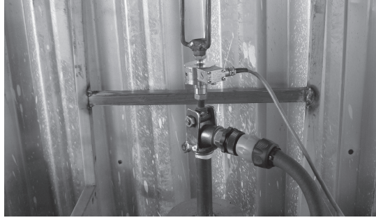
Phot. 2. Fastening of pipeline at measuring position
