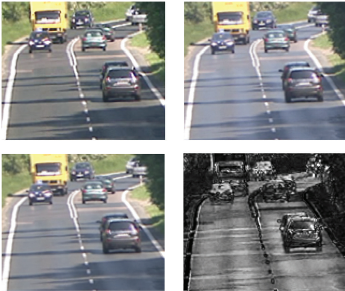
Fig.4. Reference frame: (acquired with polarisation filter 1 (left-up), acquired with polarisation filter2 (right-up), average of both polarised images and the absolute difference between them (right-down))
