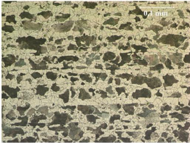
Rys. 1. Struktura stali gatunku B27 – stan dostarczenia Fig. 1. Structure of steel grade B27- state of delivery
