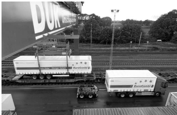
Fig. 2. Transhipment of a semi-trailer in an ITR-terminal Source: [7]
