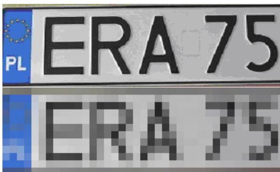
Fig. 1. Example of a high resolution image containing a fragment of a register plate and resized low resolution one Source: [own work]
