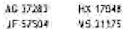
Fig. 8. Reconstructed images obtained using the super-resolution algorithm for the uniform sampling with 10% horizontal and vertical disturbance Source: [own work]
