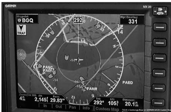
Fig.3.Example of TIS-B service on ADS-B equipped aircraft
