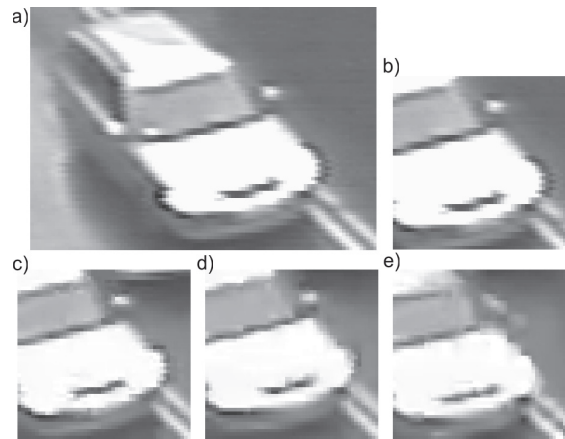
Fig.1. Video frames recovered from compressed stream – a), b) original content, c) 150, d) 500, e) 1400 compression ratios
