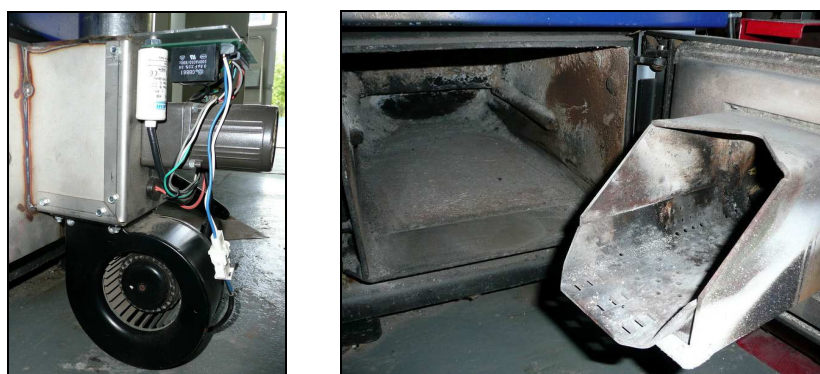
Fig.2. Furnace view: fixed-speed screw pellet dispenser; fan; air outlets
