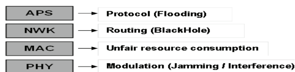
Fig. 4. Possibilities of DoS attack realisation in relation to communication layer of protocol
