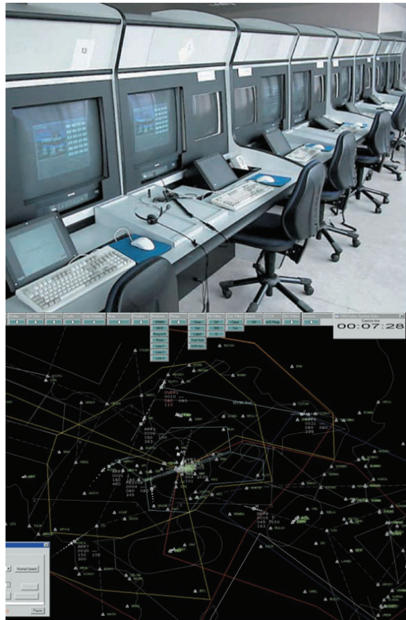
Fig. 2. Raytheon radar simulator (APP and ACC) - below radar situation display on radar indicator.
