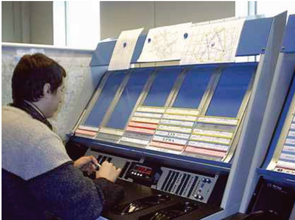
Fig.1. Procedural simulator in Aviation Training Centre ARL (PAŻP)
