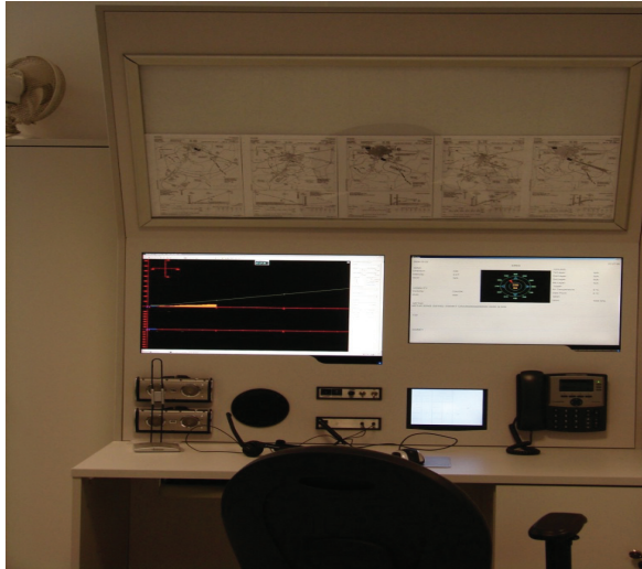
Fig. 4. Precision approach controller's position: on the right GCA 200 radar indicator, on the left weather information indicator.
