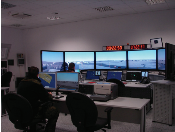
Fig. 1. Tower module of the simulating complex (phot. T. Compa)
