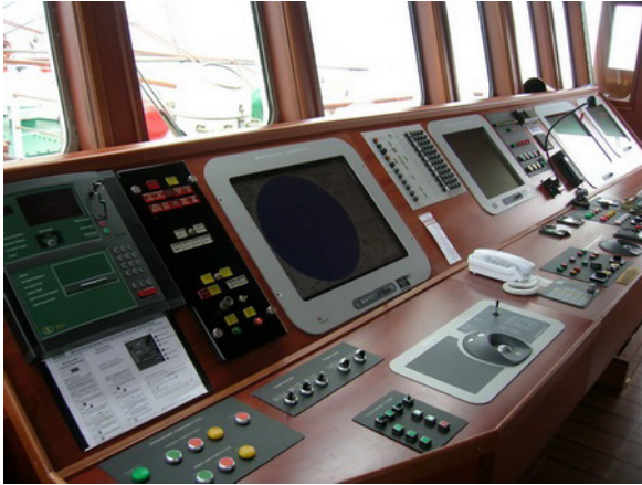
Fig. 1. Integrated navigational bridge
