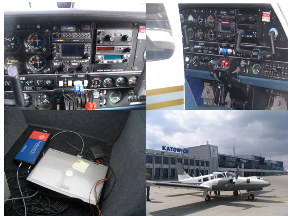
Fig. 8. GNS 430 W receiver and Septentrio receiver in the Seneca airplane and Seneca airplane on the Katowice Airport Source: [own work]
