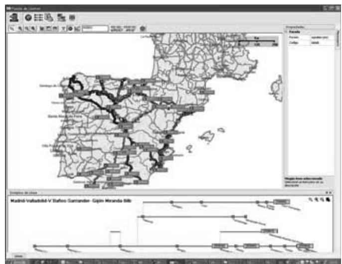
Fig.3. Display of diverse railway lines in GIS format and synoptic chart in the control centre
