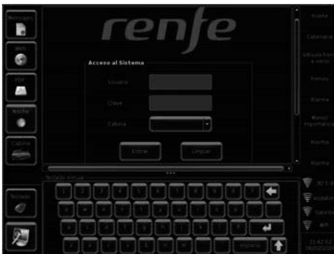
Fig.4. Driver's fleet management terminal, fitted in both cabs of the train
