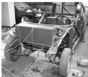
b) Fiat Seicento – model zawieszenia, suspension model
